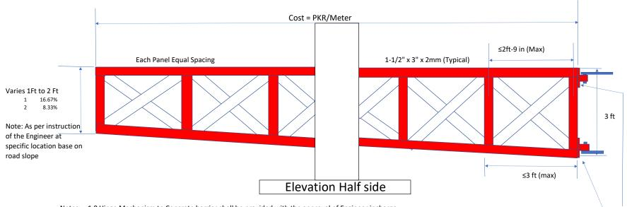
Notes: 1.0 Hinge Mechanism to Concrete barrier shall be provided with the approval of Engineer incharge.
